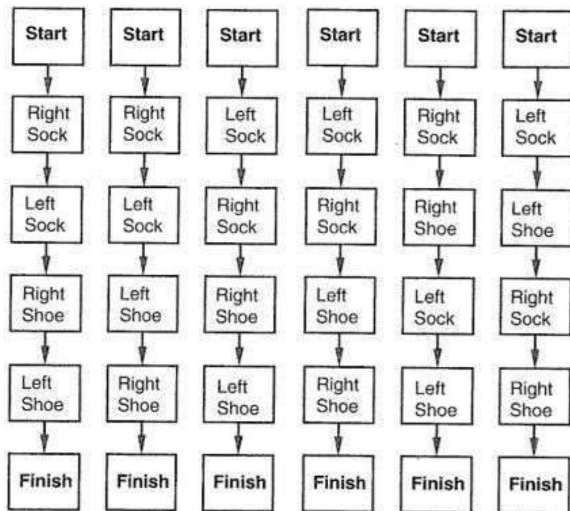
Figure 11.6 A partial-order plan for putting on shoes and socks, and the six corresponding linearizations into total-order plans.
